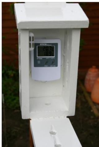
This easy-to-make weather station is intended for use with a digital thermometer. These can measure current, maximum and minimum temperatures. Some also have the facility to plug in an external thermometer which could be used to measure the grass temperature. There are some that can measure the humidity of the air to give another important weather reading. The dimensions used in this example are only a guide; adjust them if your thermometer is a different size.
