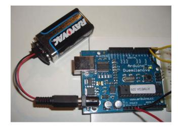
**Warning:** Watch the polarity as you connect your battery to the snap as reverse orientation could blow out your board.
