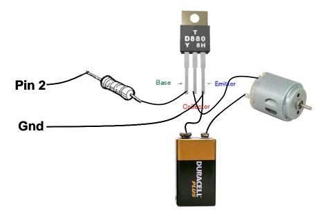
Pin 2 can be any digital I/O pin on your Arduino. Connect the minus of the battery to the emitter of the transistor (E pin) and also connect the emitter of the transistor to Gnd on the Arduino board.
