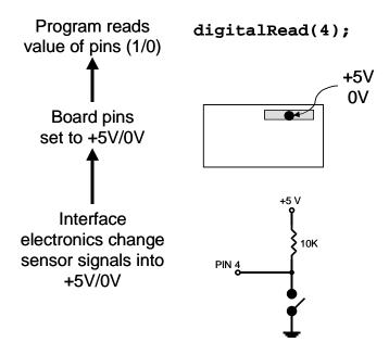
Interacting with the world has two sides. First, the designer must create electronic interface circuits that allow motors and other devices to be controlled by a low (1-10 mA) current signal that switches between 0 and 5 V, and other circuits that convert sensor readings into a switched 0 or 5 V signal. Second, the designer must write a program using the set of Arduino commands that set and read the I/O pins. Examples of both can be found in the Arduino resources section of the ME2011 web site.
