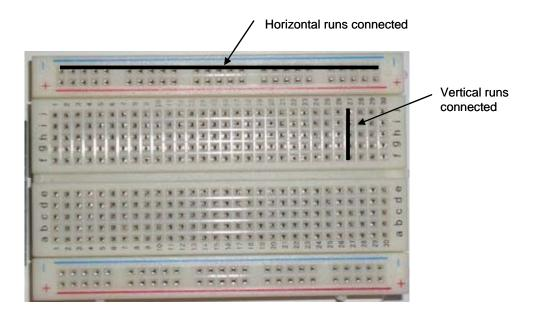
Warning: Only use solid wire on the breadboard. Strands of stranded wire can break off and fill the holes permanently.
